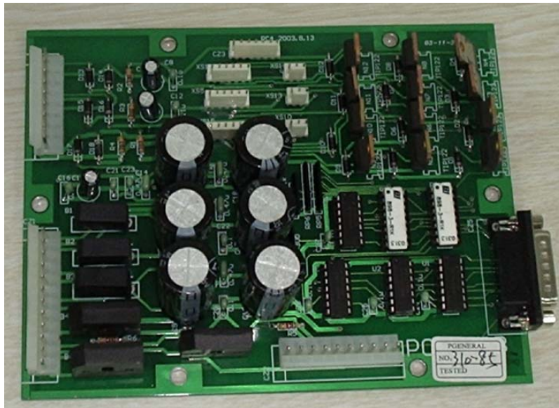
Fig.2-9 Power board PC4
