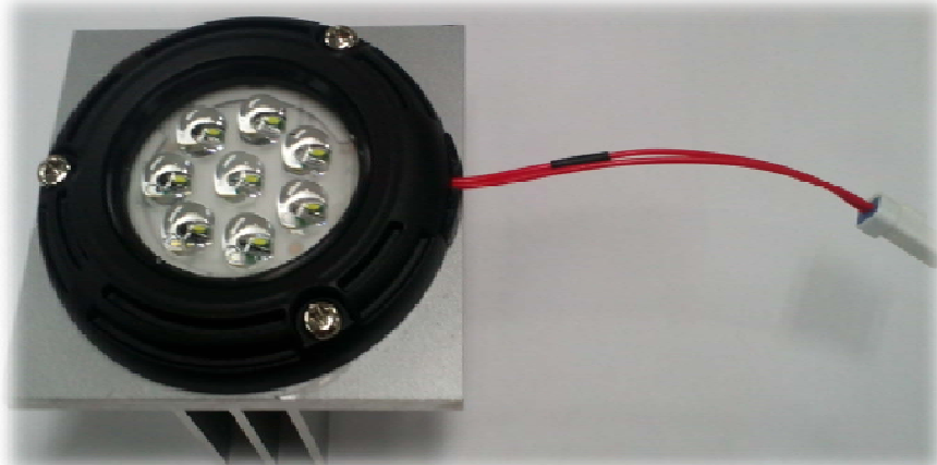
Figure.5 Assembly between Heat-sink(Al) and LED Module
