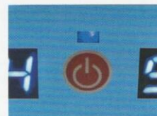
4. If the device is on and charging, the LED indicator on the device will be BLUE.
