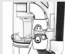
2 Raccord du tuyau
