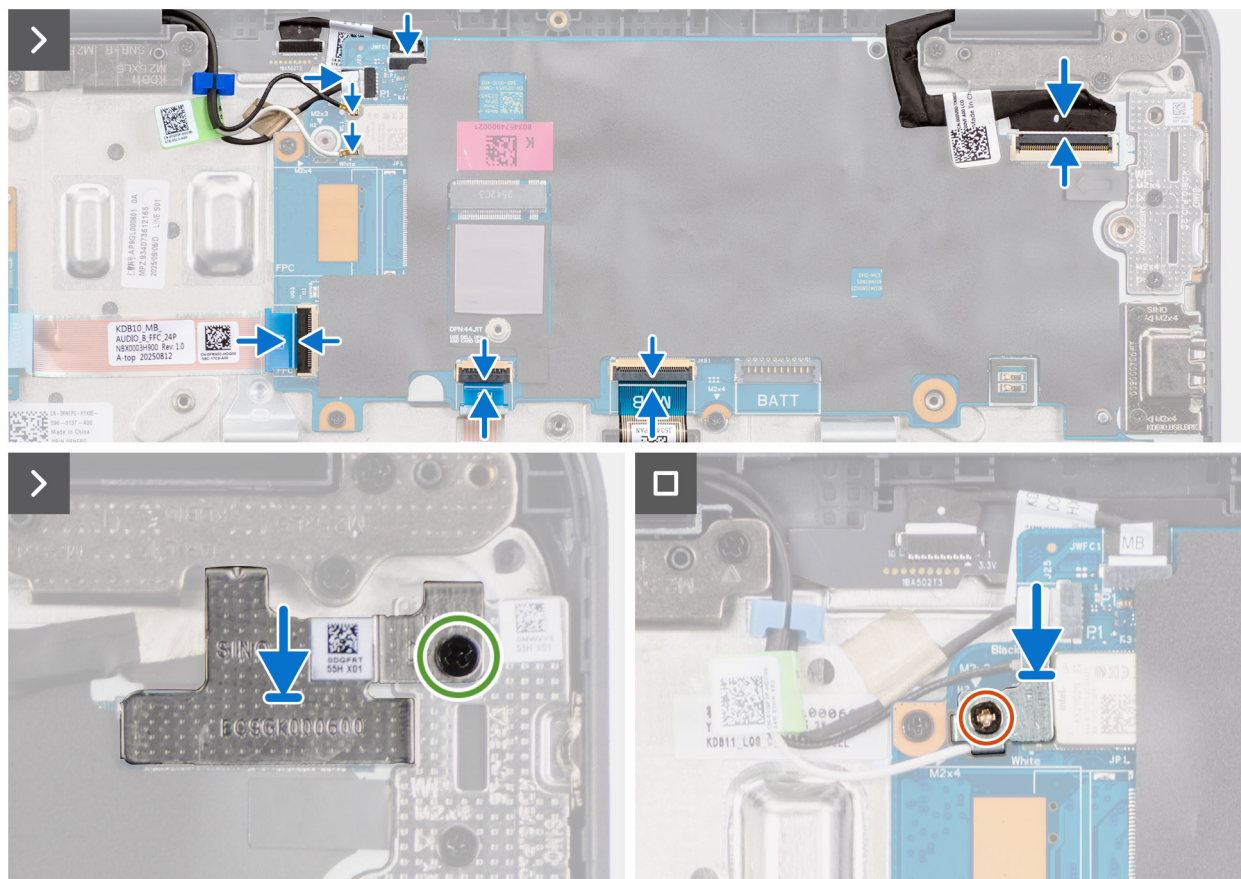
Figure 33. Installing the system board
