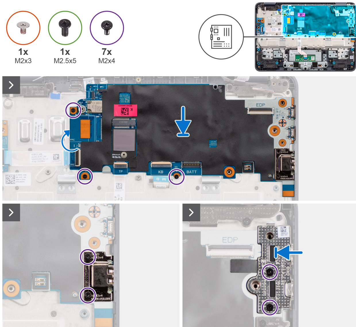
Figure 32. Installing the system board
