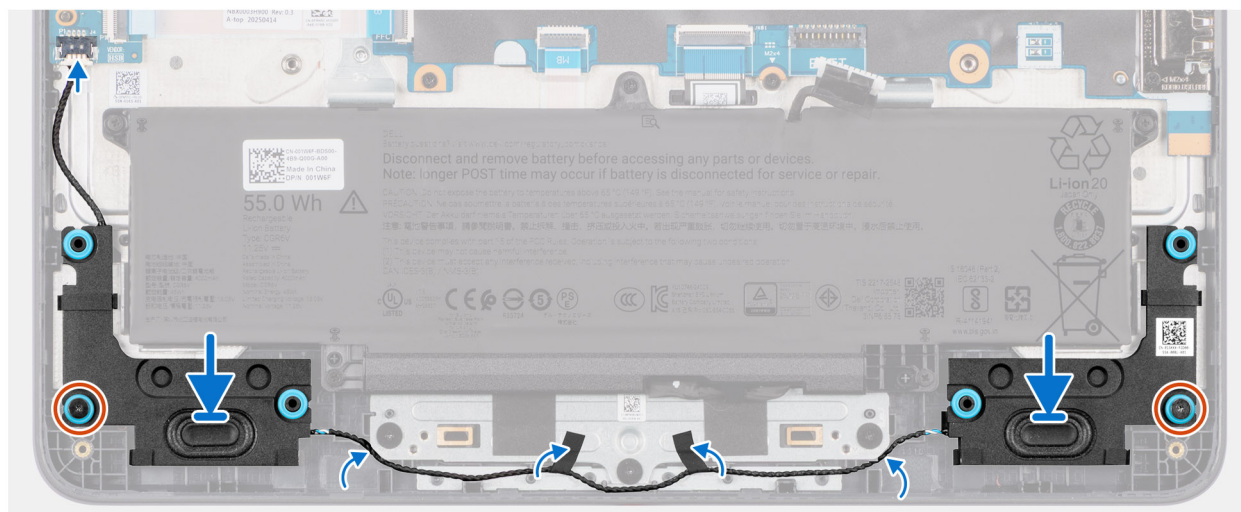
Figure 17. Installing the speakers
