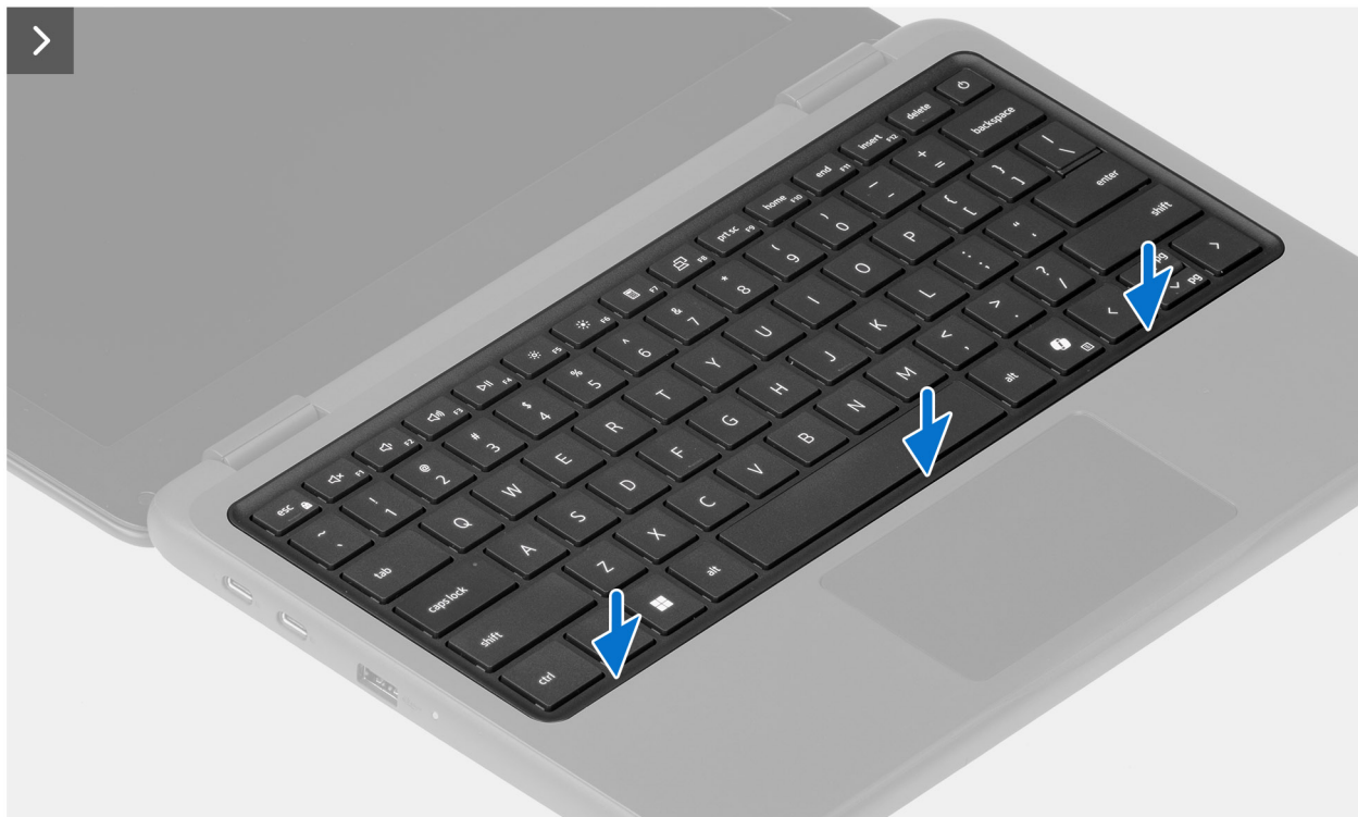
Figure 24. Installing the keyboard
