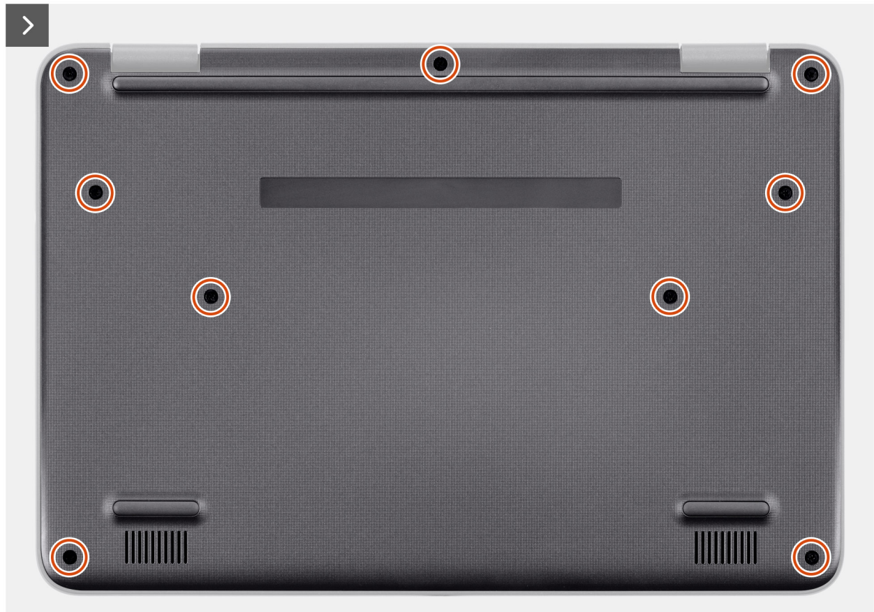
Figure 2. Loosen the base cover screws
