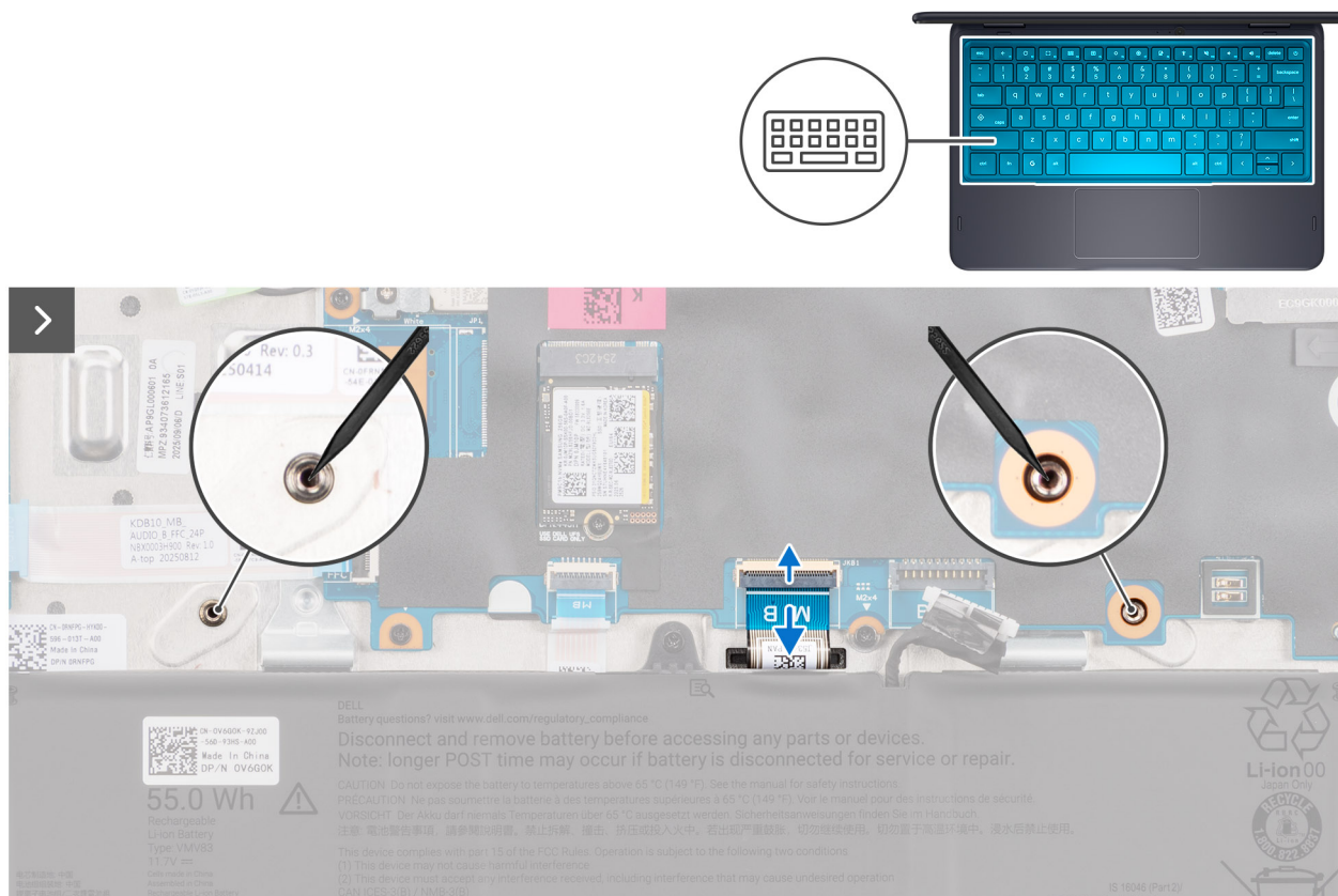
Figure 20. Disconnecting the keyboard cable
