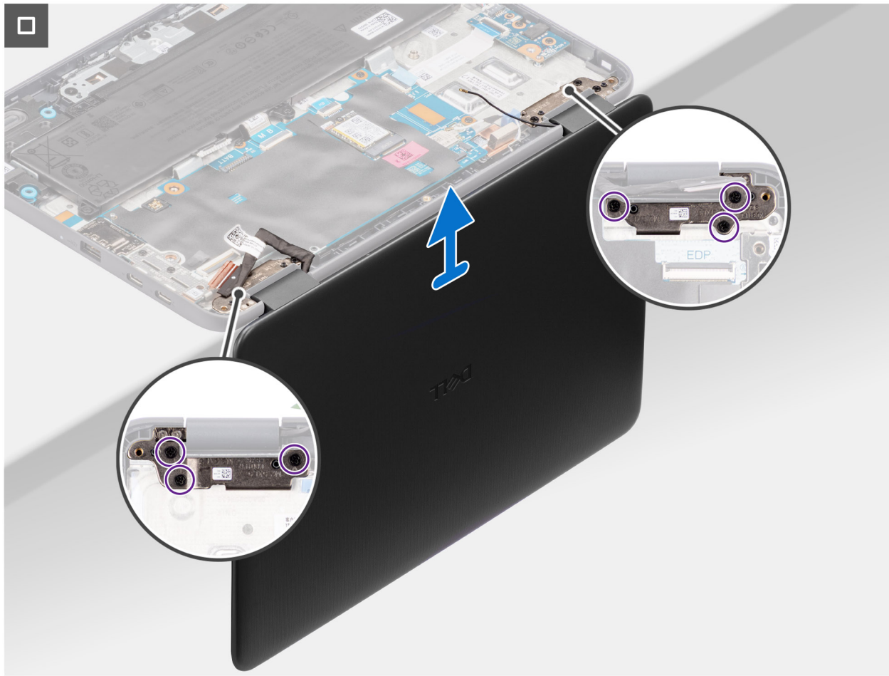
Figure 38. Removing the display assembly
