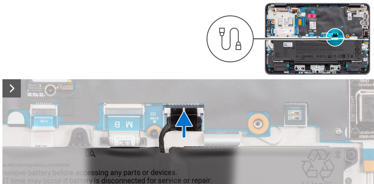
Figure 5. Connecting the battery cable
