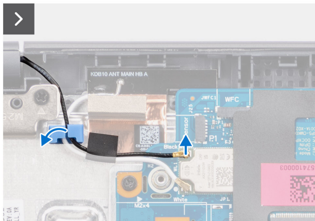
Figure 37. Removing the display assembly
