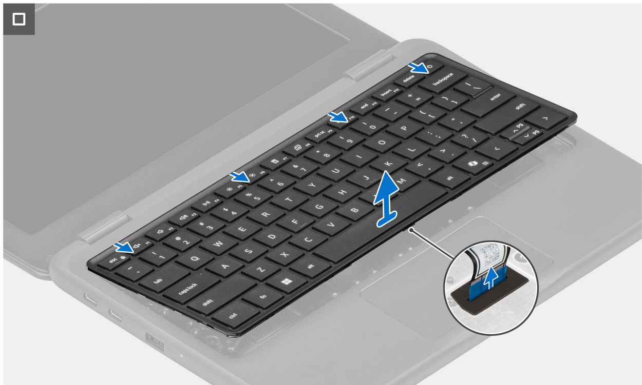
Figure 22. Removing the keyboard
