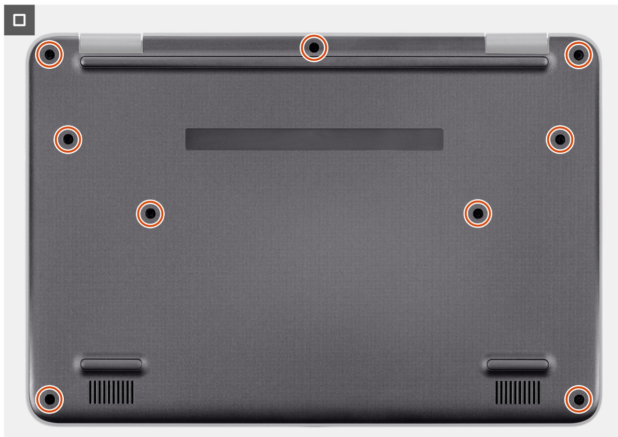
Figure 7. Tightening the base cover screws
