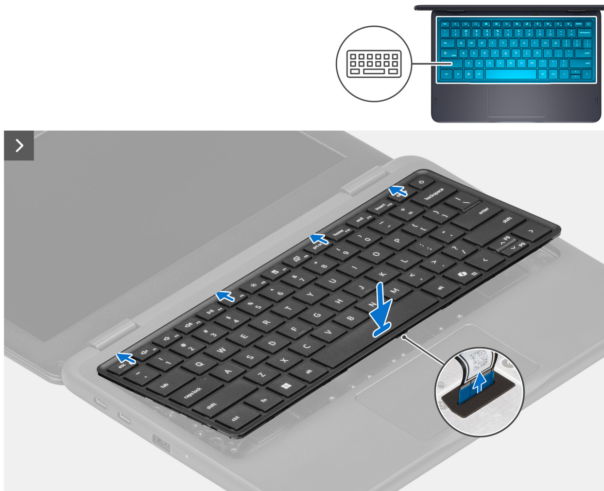
Figure 23. Inserting the keyboard cable through the opening on the palm-rest assembly and placing the keyboard on it
