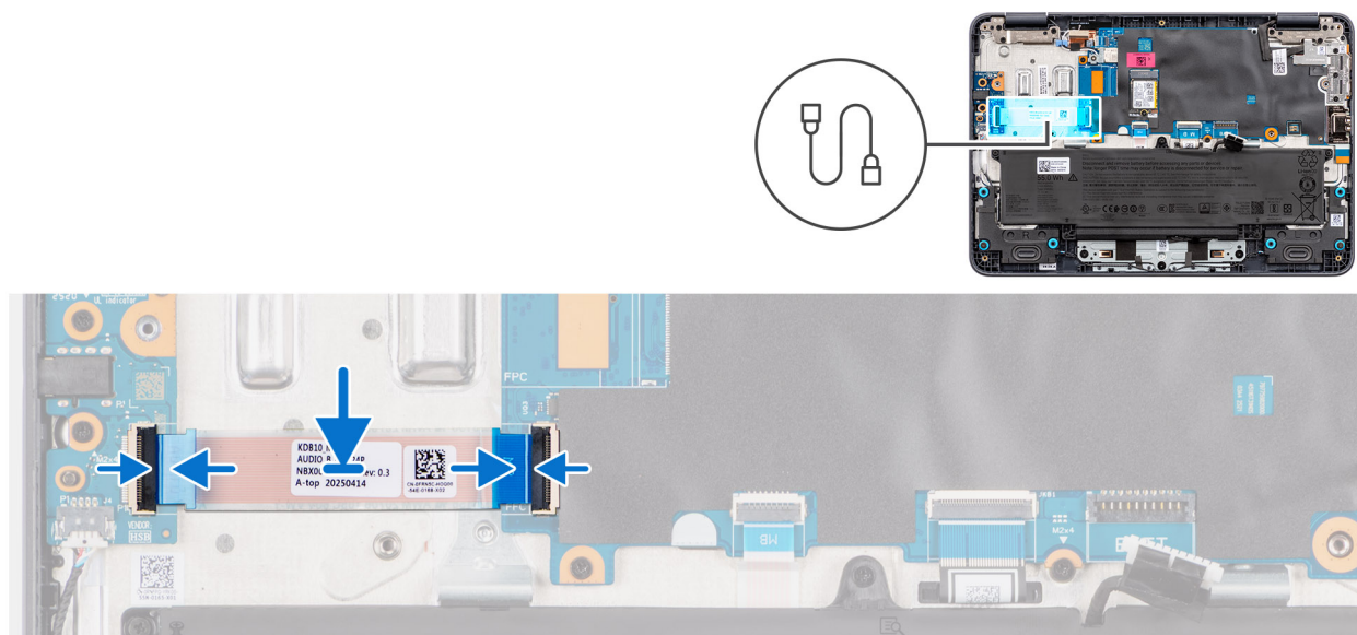
Figure 13. Installing the I/O board cable
