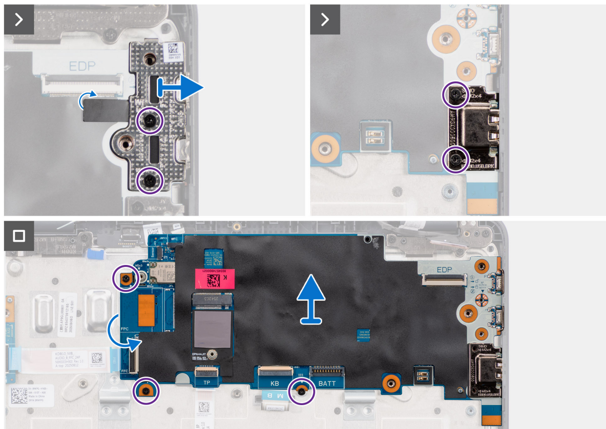
Figure 30. Removing the system board
