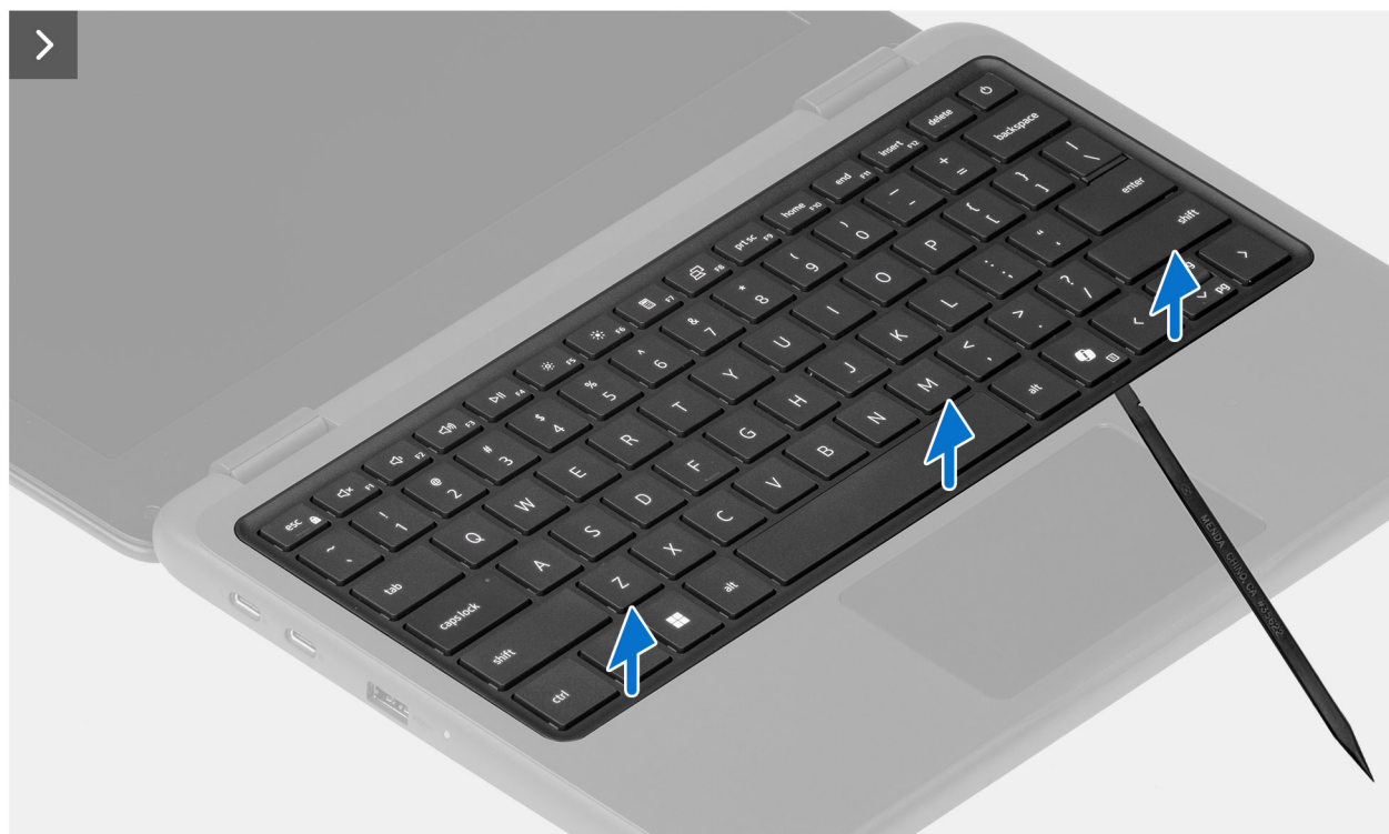
Figure 21. Releasing the keyboard with a scribe
