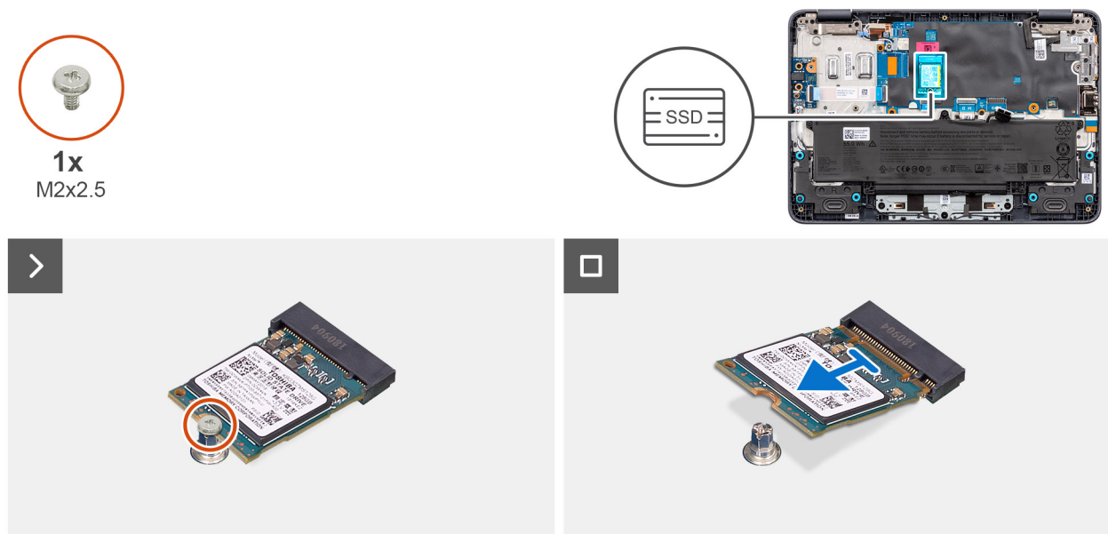
Figure 18. Removing the SSD
